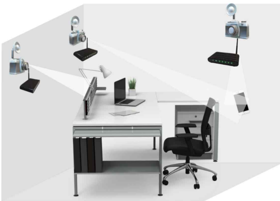
Fig . A downlink communication scenario where three candidate BSs are serving one user (mobile phone), and the other objects are potential blockages.
